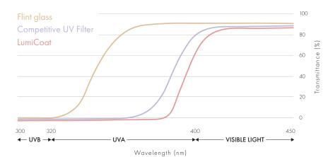
LumiCoat outperforms flint glass and the competitive UV filter by blocking both UVA and UVB rays up to 400 nm while still allowing visible light to pass through.
